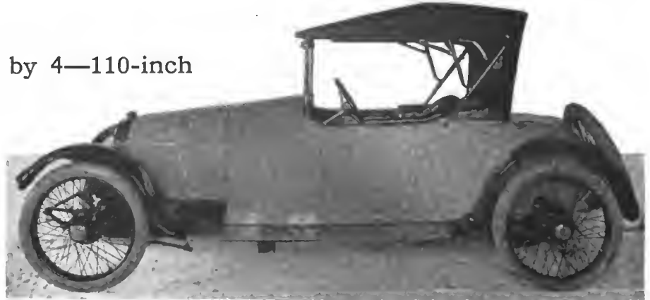
Side view of new streamline Scripps-Booth light car which sells at $775 with complete equipment including electric lighting and starting and wire wheels. The frame is over-slung instead of under-slung as shown in the illustration
